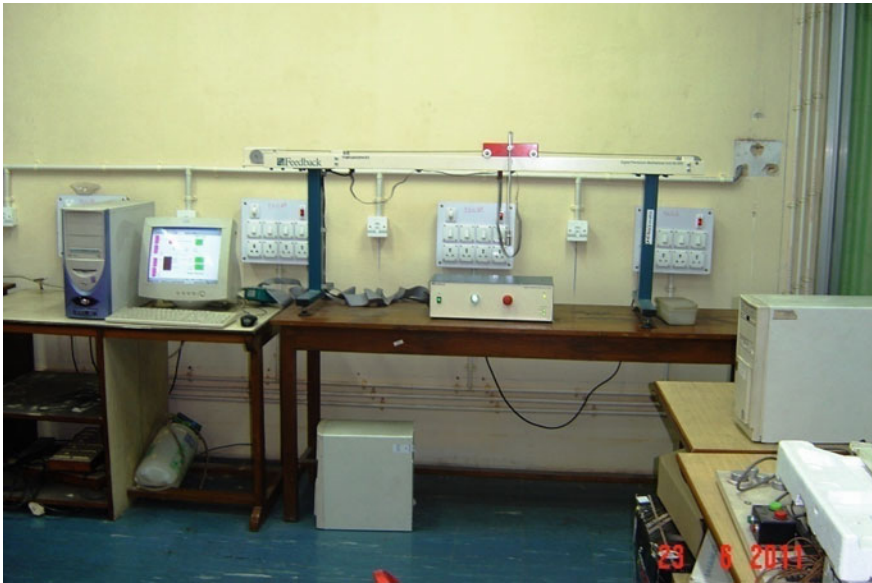
Fig. 4.37 Real-time experimental setup of single dimensional Granty crane
